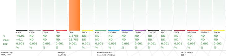
Analysis Method : SOP.T.30.031.TN & SOP.T.40.031.TN Expanded Measurement of Uncertainty: Flower Matrix d9-THC: ± 0.100, THCa: ± 0.124, TOTAL THC ± 0.112. These uncertainties represent an expanded uncertainty expressed proximately the 95% confidence level using a coverage factor k=2 for a normal distribution
